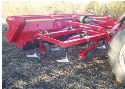
KK400s with spring-release stubble tine
