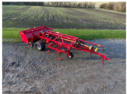
KK400s with spring-release stubble tine
